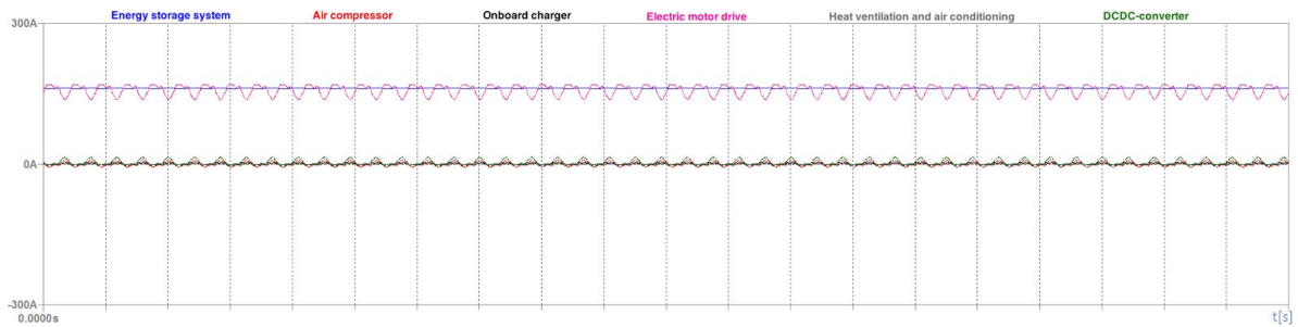
Figure 3. Simulation of current ripple in the hybrid bus with the active subsystem the electric motor drive. Current plotted between \pm 300A over time. The pink is the electric motor drive. The dark green is the DCDC- converter. The black is the onboard charger. The gray is the Heat ventilation and air conditioning. The red is the Air compressor. The blue is the Energy storage system.
